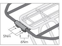
5. When all pieces are installed, adjust and straighten clamps and rails if needed. **IMPORTANT: NOW TIGHTEN ALL HARDWARE FIRMLY** (see Nm above). After installation, please check for secure fit and that everything works correctly.
