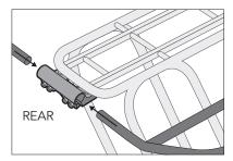
4. Insert rails all the way to the center of the clamps until they come to a stop. Loosen clamp bolts as needed for easy insertion. Install entire rail before tightening. (To see more specific rail installation instructions refer to the Rail PLUS installation manuals).
