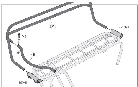
4. Insert both lower ends of left rail (A) from the left side all the way into the center of the clamps until they come to a stop. Loosen clamp bolts as needed for easy insertion. DO NOT TIGHTEN YET. Then connect rear rail (B) to the upper end of the left rail (A) as shown. Use M6 bolt, spacers and nut as shown to ensure connection between rail (A) and rail (B).
