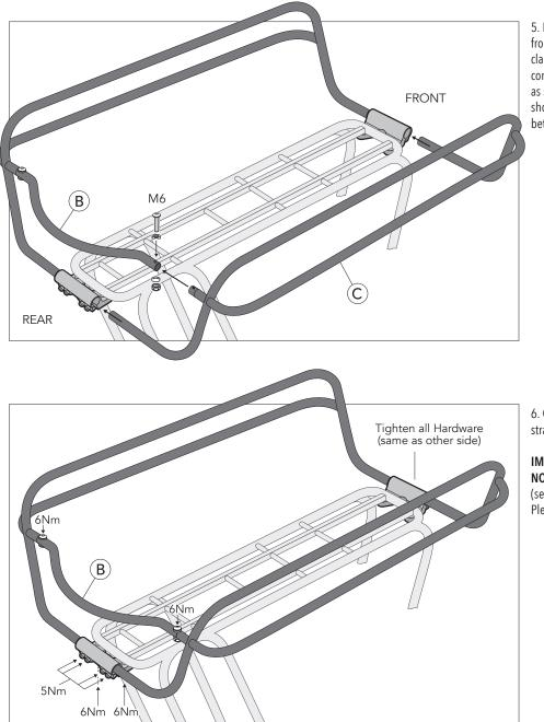
5. Insert both lower ends of right rail (C) from the right side into the center of the clamps until they come to a stop while connecting the upper end to the rear rail (B) as shown. Use M6 bolt, spacers and nut as shown to ensure secure connection between rail (B) and rail (C).
