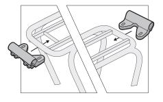
2. Place one clamp on each end of the rack (front and rear). Insert clamps from below and line up with the two fittings on the underside of the rack.
