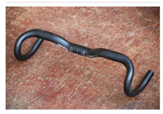
The Genetic Driser 4 handlebar has a very interesting shape and works well in quite a few disciplines thanks to its slightly flared drops and 20mm rise. Stiffness levels are high and it's a decent price for a quality alloy bar. I would like to see some kind of indentation for guiding cables and hoses, though.
