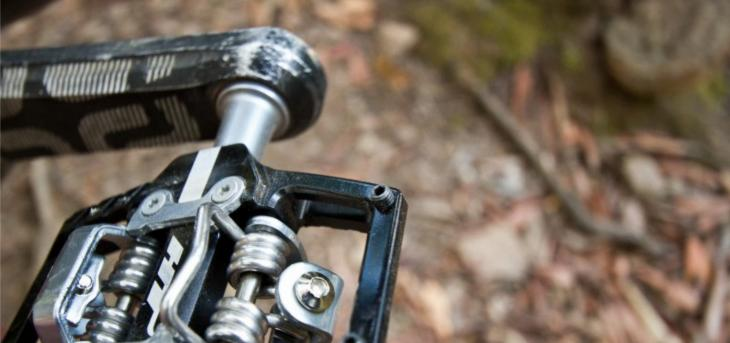
The front pins are an added bonus when it comes to finding the pedal and remaining in contact.
