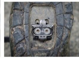
The X1 feels extremely secure thanks to the wide aluminum platform and plenty of available spring tension.
