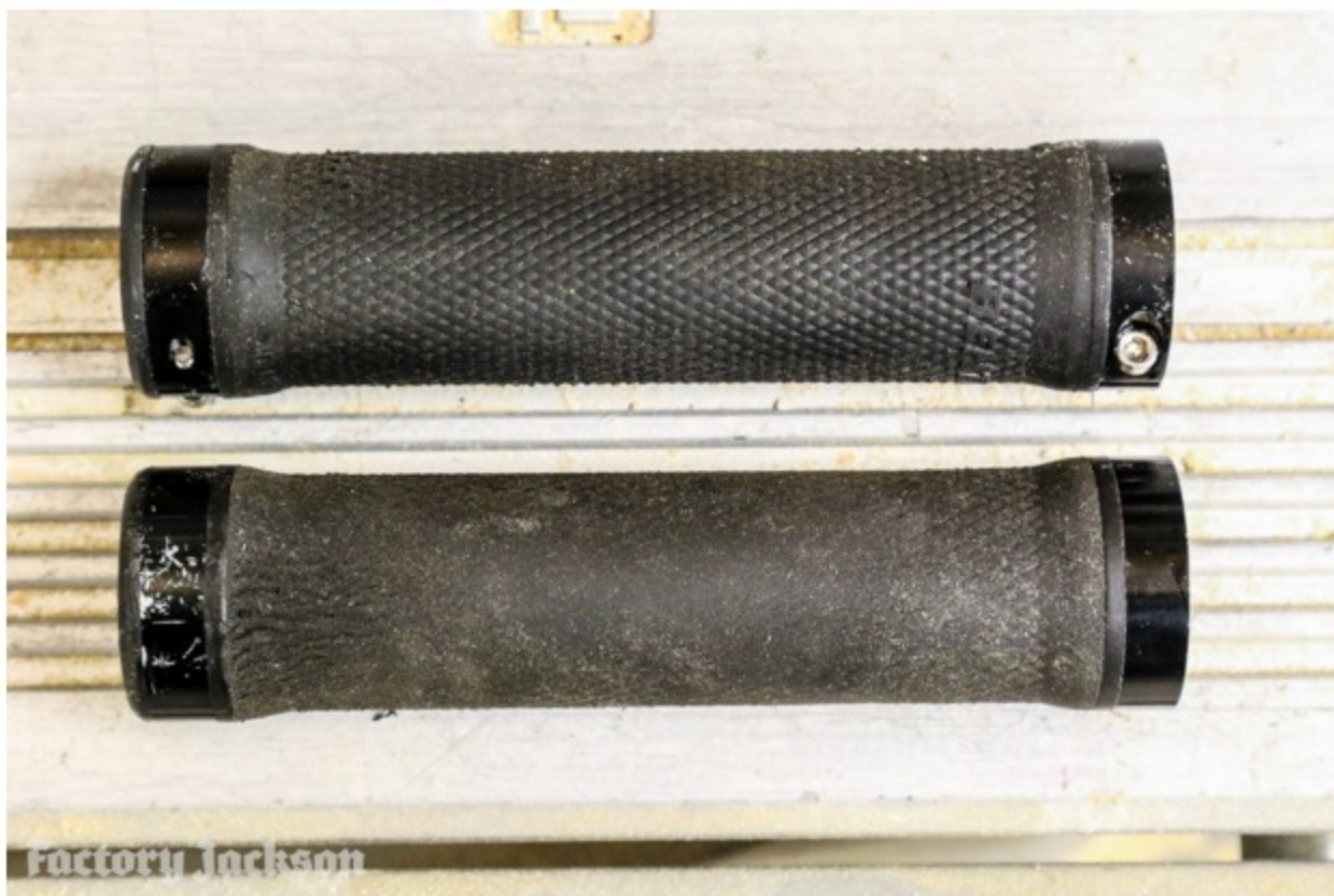
A week old Renthal Ultra Tacky lock on grip at the top, and a 17month old prototype below. The old grip feels every bit as grippy, and still absorbs a lot more trail buzz than many brand new grips.
